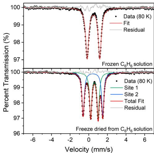
Fig. 4 (Top) Mössbauer spectrum of a flash-frozen benzene solution of **1**. Fit parameters:  $\delta = 0.50 \text{ mm s}^{-1}$ ,  $\Delta E_Q = 1.35 \text{ mm s}^{-1}$ . (Bottom) Mössbauer spectrum of the same sample, after subliming away the benzene. Fit parameters:  $\delta = 0.60 \text{ mm s}^{-1}$ ,  $\Delta E_Q = 0.80 \text{ mm s}^{-1}$  (site 1, green);  $\delta = 0.45 \text{ mm s}^{-1}$ ,  $\Delta E_Q = 2.11 \text{ mm s}^{-1}$  (site 2, blue). Both spectra were recorded at 80 K.
