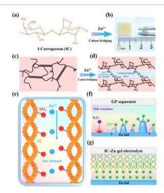
Fig. 1 (a) Chair configuration of iota-carrageenan. (b) Optical photographs of IC–Zn gel electrolyte. The proposed structures of (c) IC gel and (d) IC–Zn gel, respectively. (e) Zinc ion channel in IC–Zn gel electrolyte. Schematic illustrations of the behavior of Zn anodes with (f) ZnSO $_4$  aqueous electrolyte and (g) IC–Zn gel electrolyte in Zn deposition.
