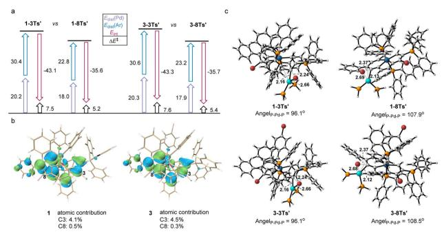
Fig. 3 (a) Distortion/interaction analysis. All energies were computed at the level B3LYP-D3/def2-TZVP/PCM(o-DCB), and are given in kcal mol<sup>-1</sup>. (b) LUMO of 1 and 3. (c) TSs for oxidative insertion into C3-Br and C8-Br.
