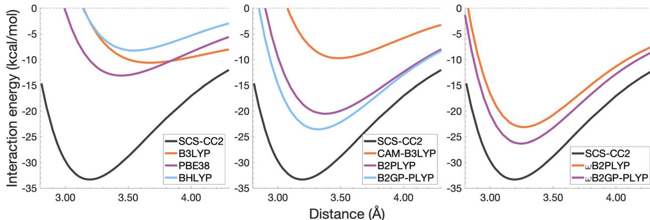
Fig. 9 Dissociation energy curves of the lowest-lying singlet excited state of the fully-stacked pyrene dimer.
