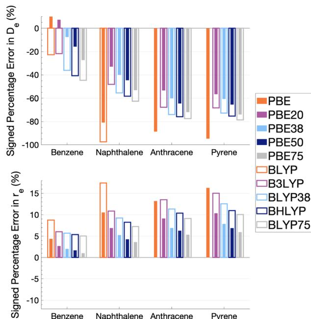
Fig. 5 Percentage error in dissociation energy ( $D_e$ , top) and equilibrium inter-monomer separation ( $r_e$ , bottom) of each excimer with respect to SCS-CC2/CBS(3,4) for varied Fock exchange with PBE and BLYP exchange-correlation functionals. BLYP results are not shown for anthracene and pyrene excimers as they gave repulsive dissociation curves.
