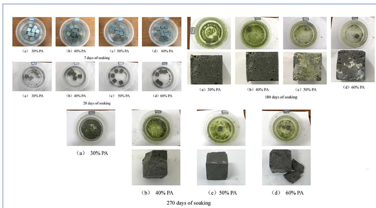
Fig. 16 Evolution of geopolymer specimens different soaking times, Pu *et al.*, *Dev. Built Environ.*, 2022.<sup>97</sup>
