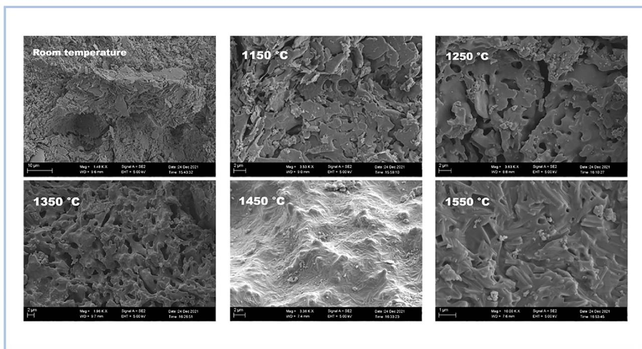
Fig. 10 SEM images of samples treated at different temperatures, Wei *et al.*, *Materials*, 2022.<sup>72</sup>
