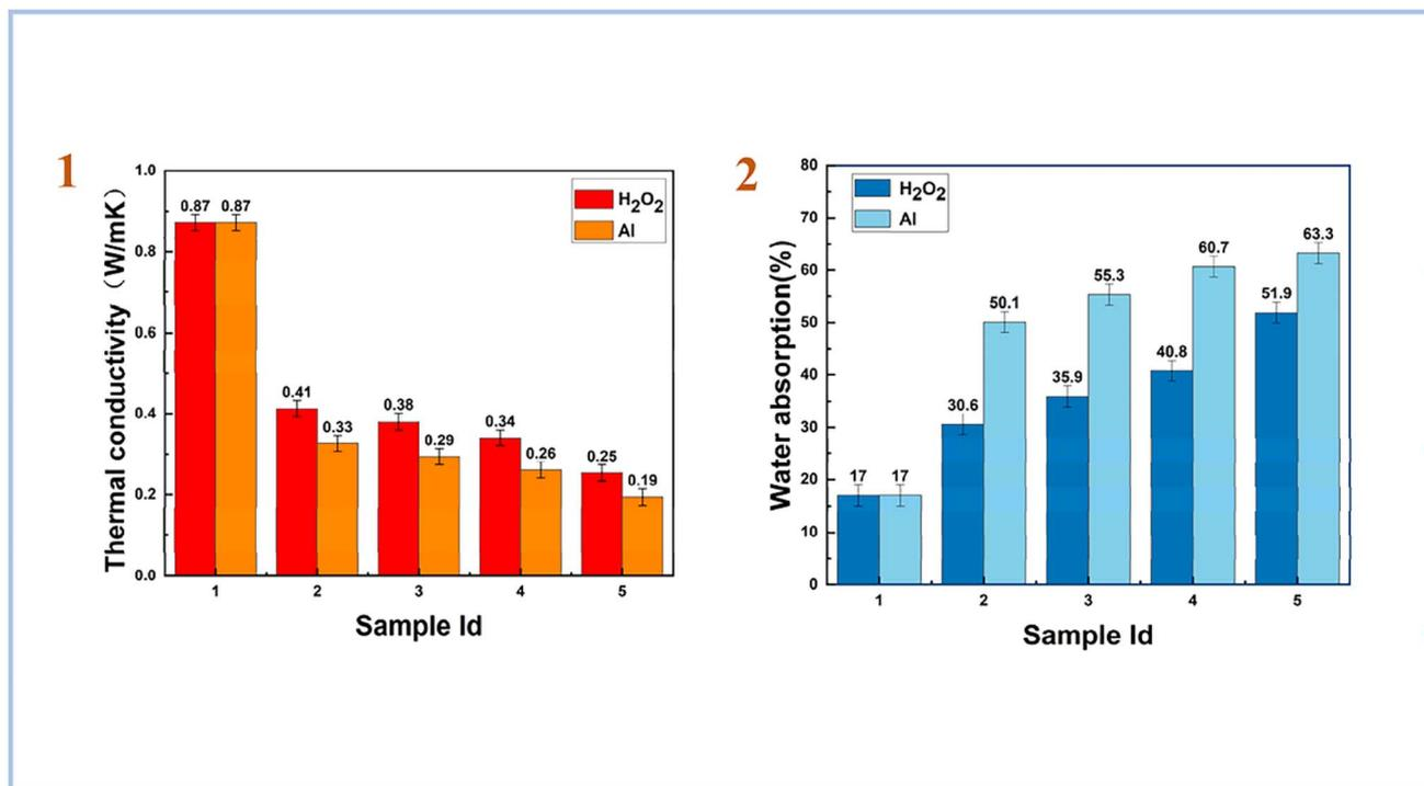
Fig. 13 (1) thermal conductivity of HMNS-FA-phosphate-based porous geopolymers; (2) water absorption (%) of HMNS-FA-phosphate-based porous geopolymers, Yang *et al.*, *Minerals*, 2023.<sup>83</sup>
