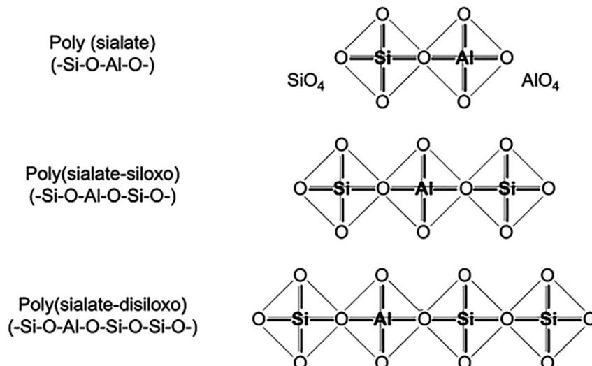
Fig. 1 Structural unit model of geopolymer with different Si/Al ratios, Davidovits *et al.*, *J. Therm. Anal.*, 2008.<sup>2</sup>
