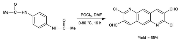
Scheme 49 Synthesis of 2,7-dichloropyrido[2,3-g]quinoline-3,8-dicarbaldehyde.
