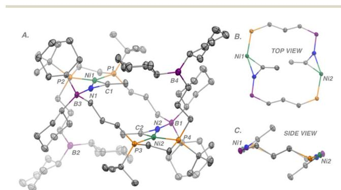
Fig. 3 (A) Molecular structure of **2**; (B) top view; (C) side view. Thermal ellipsoids are shown at the 50% probability level. Hydrogen atoms have been omitted for clarity. Selected bond distances (Å): Ni1–C1 1.236(2), Ni2–C2 1.236(2), Ni1–Ni2 6.484(8), B1–N2 1.629(2), B3–N1 1.629(2), Ni1–N1 1.907(14), Ni2–N2 1.907(14), Ni1–C1 1.856(17), Ni2–C2 1.856(17).
