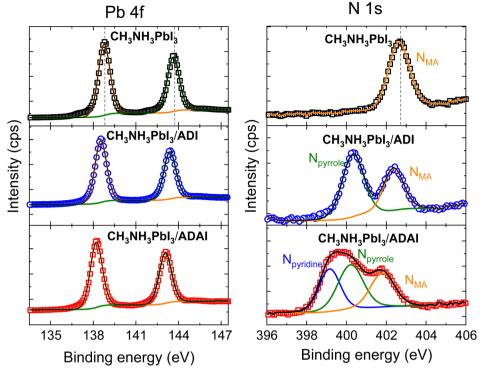
Fig. 10 Pb 4f and N 1s core level XPS spectra of bare CH<sub>x</sub>NH<sub>x</sub>PbI<sub>x</sub> and CH<sub>x</sub>NH<sub>x</sub>PbI<sub>x</sub> coated with **ADI** and **ADAI**.
