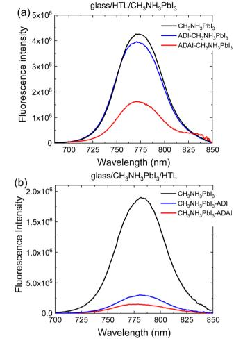
Fig. 7 Photoluminescence spectra registered by excitation of the perovskite through the HTL interface. The relative position of the HTL with respect to the perovskite is indicated
