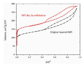
Fig. 9 Nitrogen sorption isotherms for the original layered MFI and an MFI disc (shifted vertically by  $50 \text{ cm}^3 \text{ g}^{-1}$ ).
