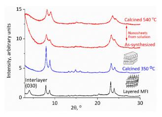
Fig. 2 XRD patterns of the as-synthesized layered MFI (bottom), calcined at 350 °C (second from bottom), and exfoliated nanosheets recovered by acidification, uncalcined, and calcined (top).
