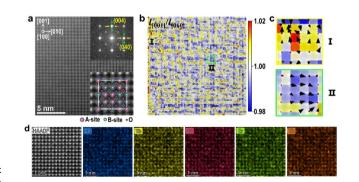
Fig. 3 (a) HAADF-STEM image along the [100] zone axis for the pyrochlore type (Yb,Tb,Gd,Dy,Er)<sub>2</sub>Ti<sub>2</sub>O<sub>7</sub> HEO with the corresponding FFT pattern in the top inset and the projected structure model in the bottom inset. (b) Lattice strain vectors overlaid on colormaps of the aspect ratios  $(l_{[001]}/l_{[010]})$  for all quadrangle units in (a). (c) Enlargements of two types of domains in (b). (d) Atomic-resolution EDS elemental maps of Gd, Tb, Dy, Er, and Yb.
