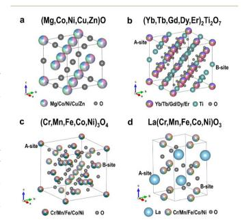
Fig. 1 Crystal structures of (a) rock-salt type (Mg,Co,Ni,Cu,Zn)O, (b) pyrochlore type (Yb,Tb,Gd,Dy,Er)<sub>2</sub>Ti<sub>2</sub>O<sub>7</sub>, (c) spinel type (Cr,Mn,Fe,Co, Ni)<sub>3</sub>O<sub>4</sub>, and (d) perovskite type La(Cr,Mn,Fe,Co,Ni)O<sub>3</sub>.
