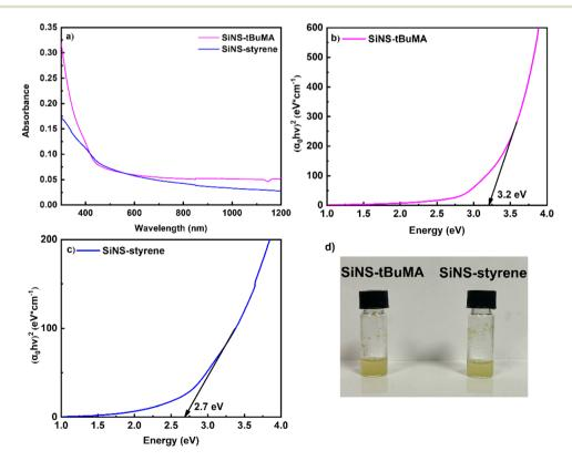
Fig. 2 (a) UV-Vis-NIR absorption spectra of SiNS-tBuMA and SiNS-styrene dispersions in toluene. Tauc plot diagrams of (b) SiNS-tBuMA and (c) SiNS-styrene for direct optical transitions. (d) Photos of SiNS-tBuMA and SiNS-styrene dispersed in toluene.
