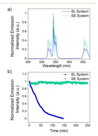
Fig. 3 (a) Normalized upconversion emission spectra of the SL and SE systems under 800 nm excitation. (b) Emission intensity of the  $^4\text{S}_{3/2}$ ,  $^2\text{H}_{11/2} \rightarrow ^4\text{I}_{15/2}$  transition of Er<sup>3+</sup> in the SL (blue) and SE (green) systems as a function of time under 800 nm excitation.
