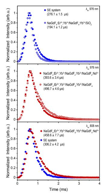
Fig. 4 Upconversion lifetimes of the  $^2H_{11/2} \rightarrow ^4I_{15/2}$  transition of Er $^{3+}$  in (a) the SE system (filled circles) and NaGdF $_4$ :Yb $^{3+}$ ,Er $^{3+}$ /NaGdF $_4$ :Yb $^{3+}$  LnUCNPs coated with unfunctionalized silica (outlined circles) under 976 nm excitation. (b) NaGdF $_4$ :Yb $^{3+}$ ,Er $^{3+}$ /NaGdF $_4$ :Yb $^{3+}$ /NaGd
