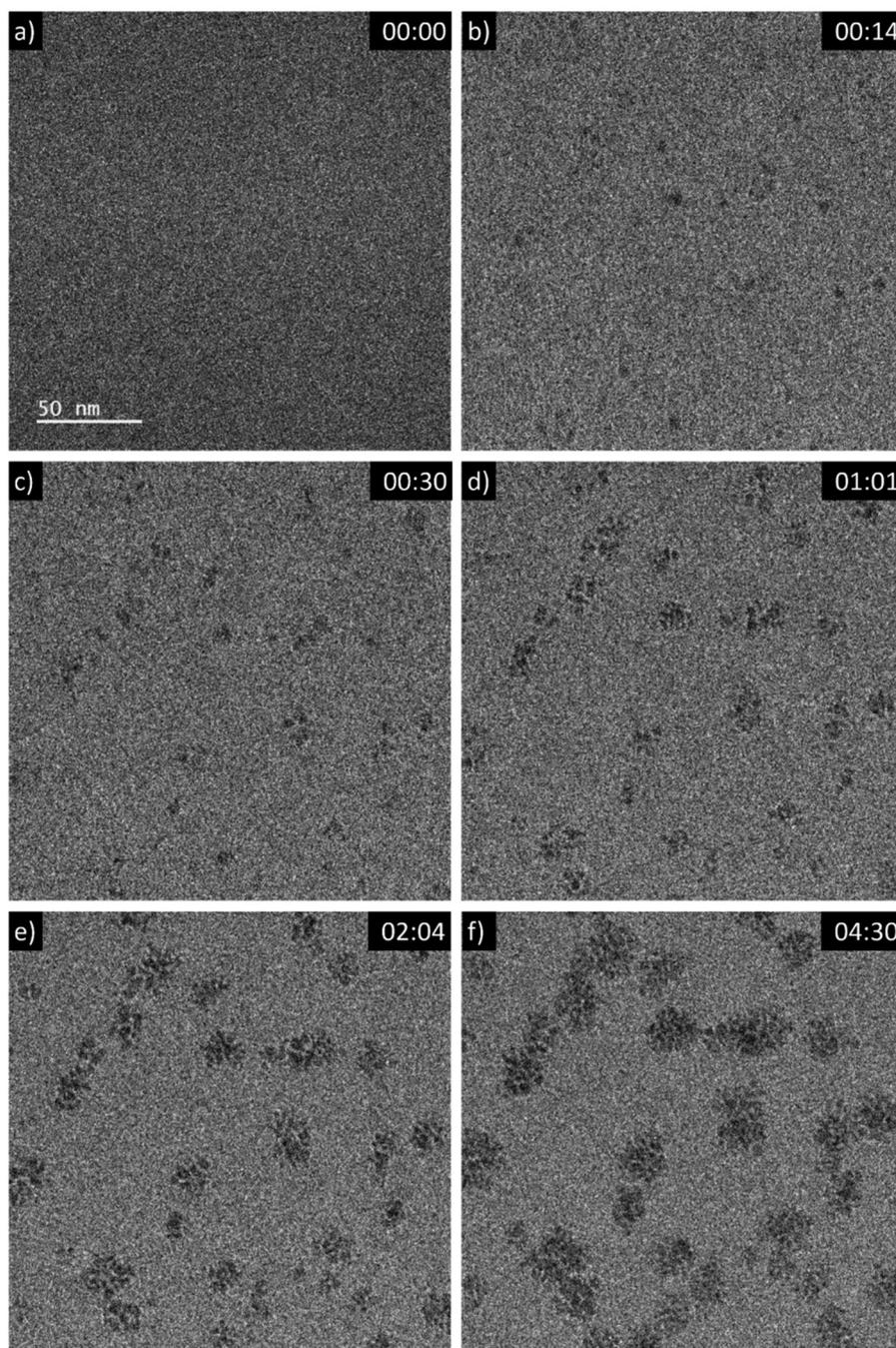
**Fig. 1** Sequential images from an *in situ* LP-TEM movie showing the formation of aggregates (see video "V01\_LP-TEM\_CeO<sub>2</sub>-nanoparticles.avi", time given as mm:ss). A dose rate of  $16.7 \times 10^6 \text{ Gy s}^{-1}$  is applied.
