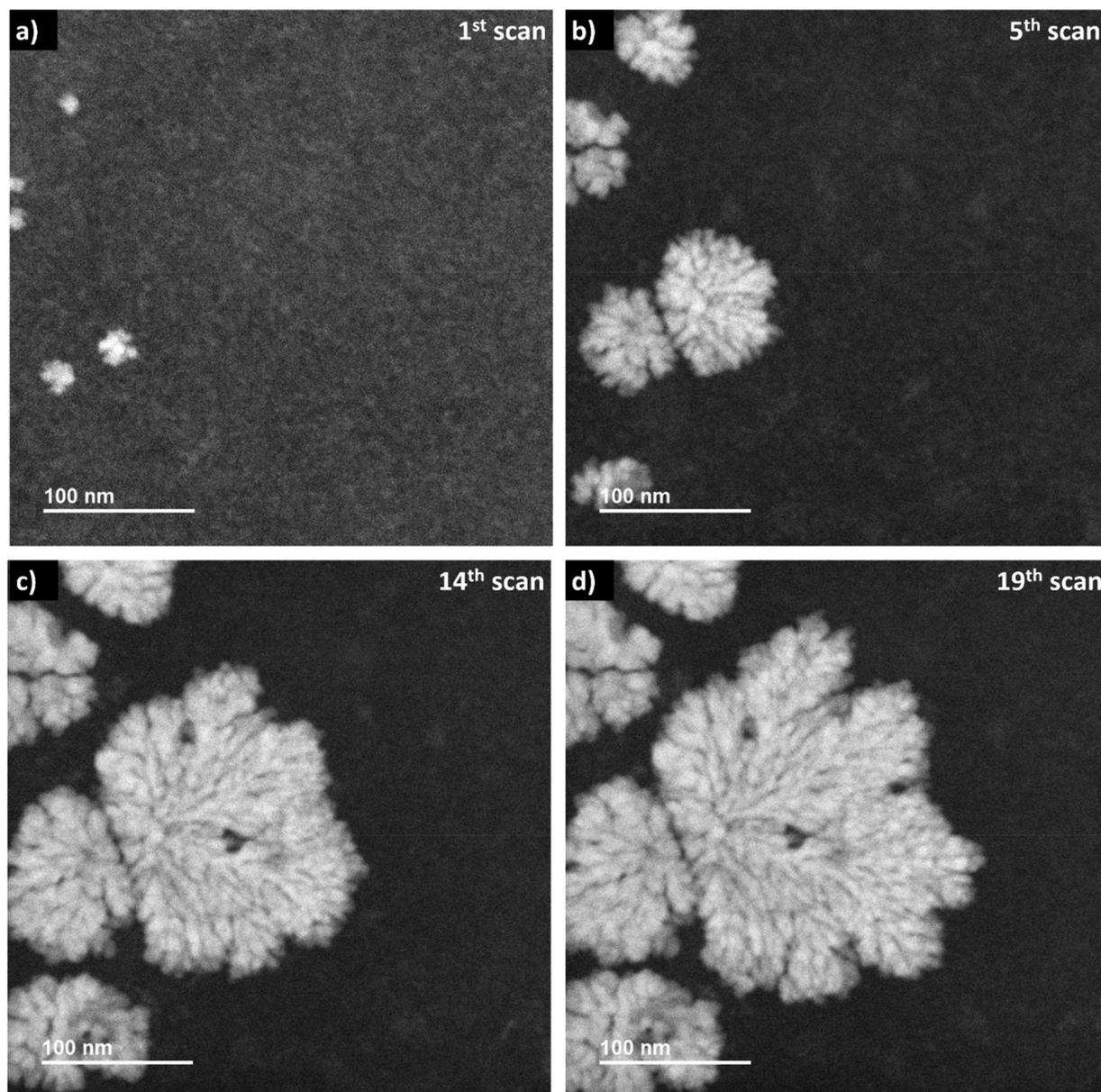
**Fig. 5** Sequential *in situ* ADF imaging in LP-STEM. An average dose rate of  $5.9 \times 10^6 \text{ Gy s}^{-1}$  is applied. (a) Already within the first scan, the aggregates become visible. (b) Continuous growth of aggregates while no formation of the additional ones is observed. (c) The appearance of the growing aggregates changes from isotropic to branched structures. (d) Further development of branched structures to larger sizes (video "V03\_LP-STEM\_CeO<sub>2</sub>-nanoparticles.avi").
