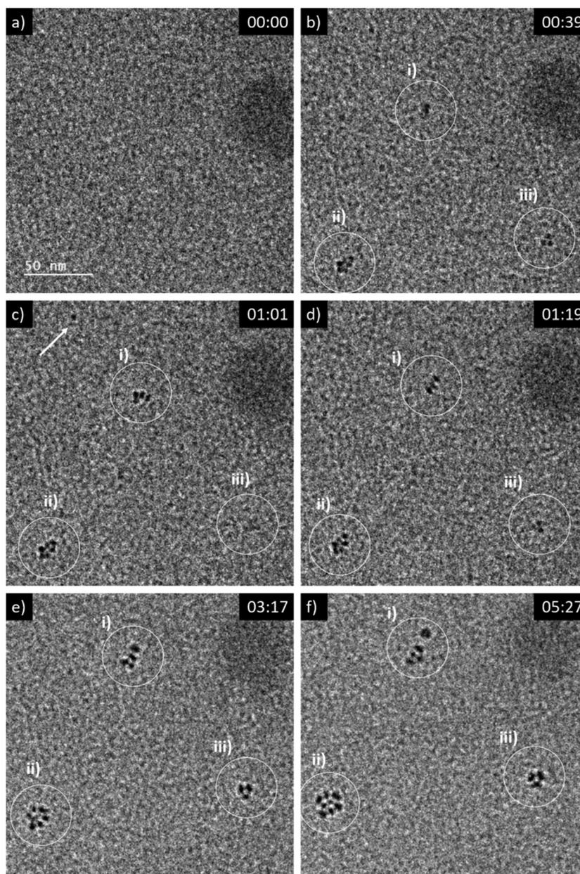
**Fig. 2** Sequential images from an *in situ* LP-TEM movie showing (a)–(b) formation and (c)–(f) arrangement of primary particles when a dose rate of  $16.7 \times 10^6 \text{ Gy s}^{-1}$  is applied. Primary  $\text{CeO}_2$  particles can be resolved and evaluated quantitatively, because of lower thickness of the liquid in comparison to Fig. 1. (See also according video “V02\_LP-TEM\_CeO<sub>2</sub>-nanoparticles”; time given as mm:ss).
