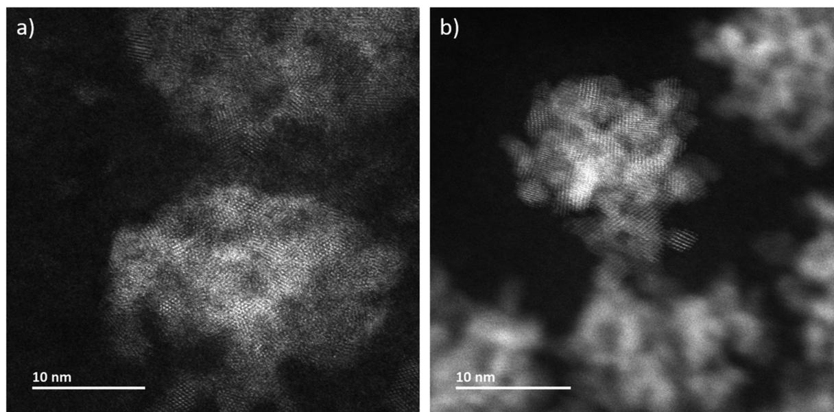
Fig. 3 ADF-STEM images of CeO<sub>2</sub> grown (a) in LP-TEM (dose rate  $16.7 \times 10^6 \text{ Gy s}^{-1}$ ) and (b) under steady-state gamma radiolysis.
