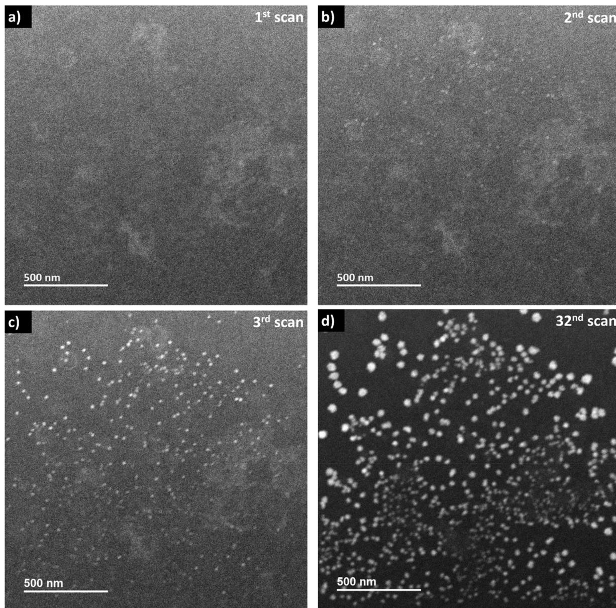
**Fig. 6** Sequential *in situ* ADF imaging in LP-STEM. An averaged dose rate of  $2.4 \times 10^5 \text{ Gy s}^{-1}$  is applied. (a) Initial scan. (b) Nano-sized aggregates become visible in the second scan and (c) their contrast increases during exposure. (d) The projected size of the aggregates increases constantly while almost no new ones are formed. (see video "V04\_LP-STEM\_CeO<sub>2</sub>-nanoparticles.avi").
