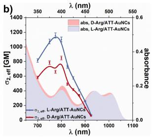
Fig. 2 (a) Two-photon circular dichroism (blue and red dots and lines, left and bottom axes) correlated with one-photon dissymmetry factor (blue and red areas, right and upper axes). (b) Two-photon brightness spectra of L-Arg/ATT-AuNCs and D-Arg/ATT-AuNCs (blue and red dots and lines, left and bottom axes) correlated with absorption of those nanoclusters(blue and red areas, right and upper axes).
