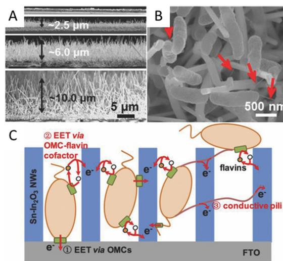
**Fig. 3** (A) Cross-section SEM images of the flat FTO film and SINW/FTO with the nanowire lengths of 2.47, 5.80, and 9.85 μm. (B) SEM images of SINW/FTO electrodes integrated with microbes of *S. loihica* PV-4 after 25 h electrochemical culture at 0.2 V. The red arrows mark the pili grown among cells. (C) Cartoon illustrating the active EET pathways on the SINW/FTO electrode. Reproduced from ref. 133 with permission from Wiley Online Library, Copyright 2018.
