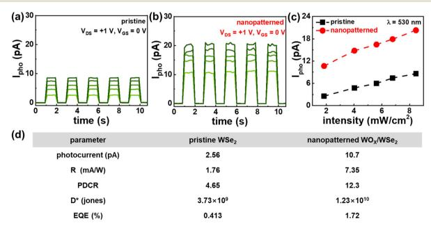
Fig. 4 Time-dependent photocurrent characteristics of the (a) pristine and (b) nanopatterned WSe<sub>2</sub> photodetector at varying optical intensities (530 nm wavelength). (c) Photocurrent at different optical intensities. (d) Optoelectronic parameters under the bias conditions of  $V_{DS}$  = +1 V and  $V_{GS}$ = 0 V considering the exposure of 530 nm with a light power density of 1.8 mW cm $^{-2}$ .
