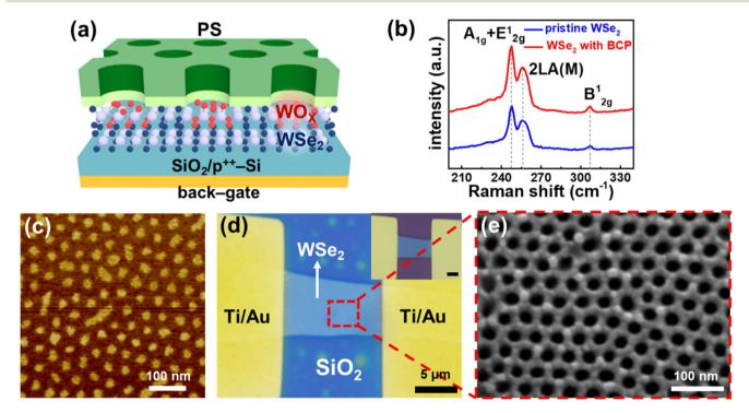
Fig. 2 (a) Schematic of the 3D WSe<sub>2</sub> homojunction with nanoporous PS. (b) Micro-Raman spectra of the pristine and BCP-patterned WSe<sub>2</sub>. (c) AFM phase image of cylinder-forming PS-b-PMMA BCP thin films on the WSe<sub>2</sub> flake. (d) Optical microscopy of the WSe<sub>2</sub> photodetector. (e) SEM images of nanoporous BCP patterns on the WSe2 photodetector.
