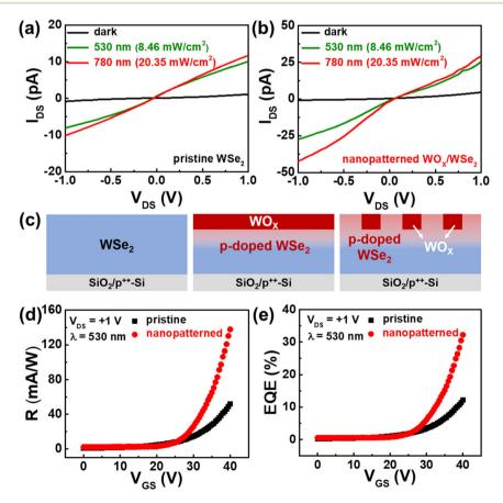
Fig. 3 Current-voltage characteristics of the (a) pristine and (b) nanopatterned WSe<sub>2</sub> device under different irradiation conditions (dark, and 530 nm and 780 nm wavelengths). (c) WSe2 without a junction (left), WSe2 with a planar junction (middle), and WSe2 with a 3D nanostructured junction (right). (d) Responsivity (R) and (e) external quantum efficiency (EQE) at varying values of  $V_{GS}$ .
