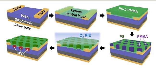
Fig. 1 Fabrication of the self-powered WSe<sub>2</sub> photodetector with the 3D nanostructured homojunction using the BCP nanolithography process.
