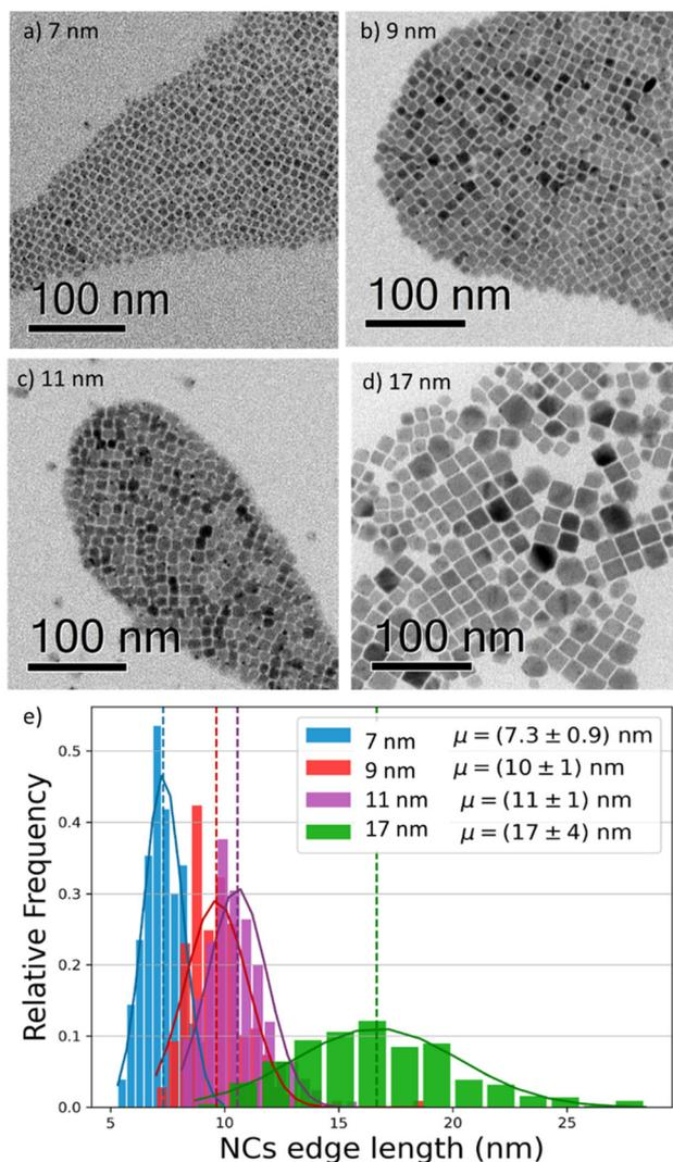
**Fig. 1** (a–d) Bright field transmission electron microscopy (TEM) images of four different CsPbI<sub>3</sub> NCs, revealing their cubic shape and sizes of 7, 9, 11, and 17 nm. The solutions have low polydispersity and narrow size distribution. (e) Size distribution histogram of the imaged NCs (statistics: 200 per size), showing narrow distributions ( $\pm 1$  nm) for the smaller sizes, and a broader distribution ( $\pm 4$  nm) for the 17 nm NCs.
