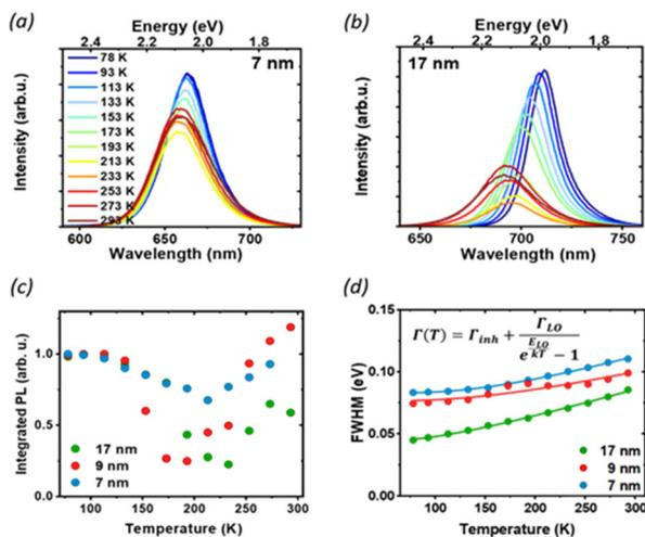
**Fig. 3** Temperature-dependent photoluminescence: PL spectra of 7 nm (a) and 17 nm (b) NCs as a function of temperature, under CW excitation at 405 nm. (c) Integrated PL intensity, normalized to the value at 77 K: the decrease in luminescence and subsequent recovery as the temperature is increased suggests the presence of non-radiative states that can be accessed at higher temperatures. (d) Temperature dependence of the PL FWHM and the corresponding fit with eqn (1).
