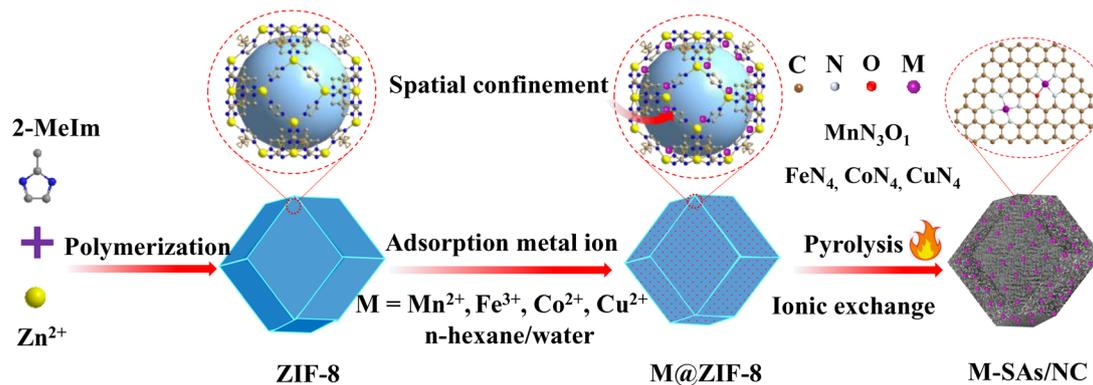
**Scheme 1** Schematic illustration of the synthesis process of metal–N species embedded in the porous N-doped porous carbon (M–SAs/NC) composite. Brown, purple, red, and white balls represent C, metal atoms, O, and N, respectively.
