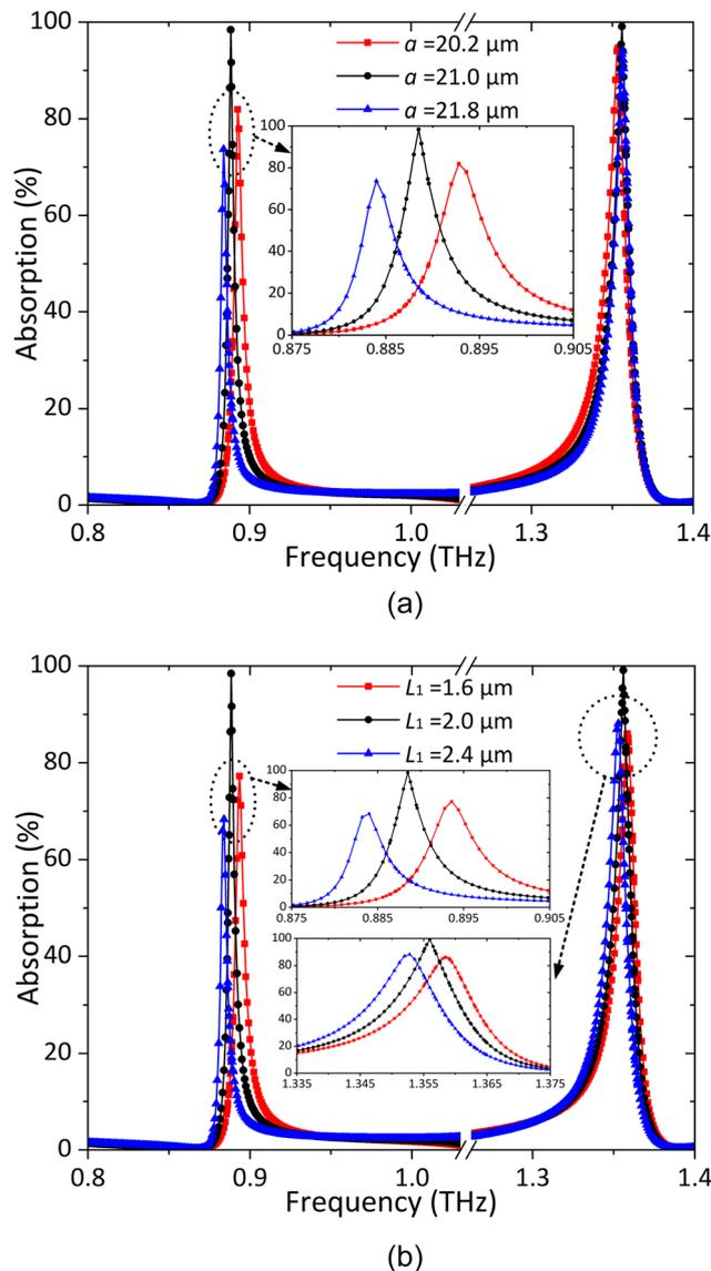
Fig. 5 Absorption spectra of the metamaterial absorber under normal TE polarization with (a) parameter  $a$  ranging from 20.2 to 21.8  $\mu\text{m}$ , (b) parameter  $L_1$  changing from 1.6 to 2.4  $\mu\text{m}$ , (c) parameter  $L_2$  shifting from 23.3 to 24.9  $\mu\text{m}$ , (d) parameter  $W_1$  increasing from 0.2 to 1.8  $\mu\text{m}$  and (e) parameter  $W_2$  growing from 1.5 to 2.5  $\mu\text{m}$ .
