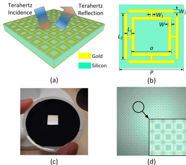
**Fig. 1** (a) Illustration of the dual-band terahertz metamaterial absorber. (b) Geometry of the metamaterial unit cell structure. (c) Photograph and (d) microscopy image of the fabricated metamaterial absorber.
