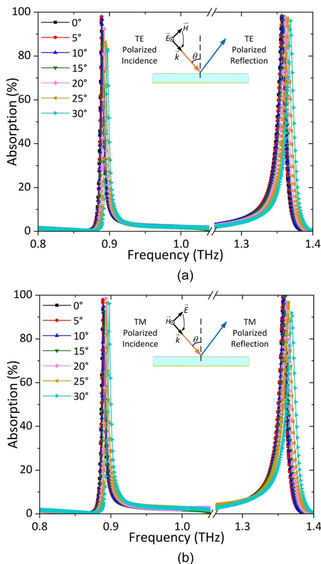
Fig. 6 Absorption performance of the metamaterial absorber with a change in the incident angle from  $0^\circ$  to  $30^\circ$  of the (a) absorption spectra under TE polarized incidence, (b) absorption spectra under TM polarized incidence, (c) Q-factors under TE polarized incidence, and (d) Q-factors under TM polarized incidence. (e) Absorption spectra with a shifting polarization angle from  $0^\circ$  to  $90^\circ$ .
