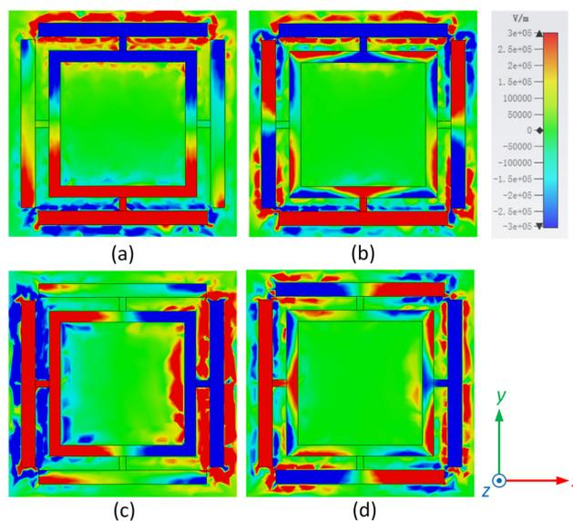
Fig. 4 Simulated distributions of the  $z$ -component electric fields of the proposed metamaterial absorber unit cell at resonant frequencies. Distributions at (a) 0.89 THz and (b) 1.36 THz under normal TE polarized incidence. (c) and (d) Distributions at 0.89 THz and 1.36 THz under normal TM polarized incidence, respectively.
