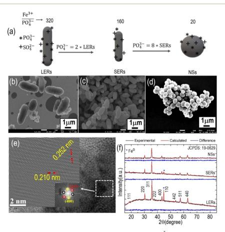
Fig. 1 (a) Schematic of the formation process of nanospheres (NS) through reduction in  $PO_4^{3-}$  concentration compared to the LERs and SERs; (b-d) FESEM image of reduced LERs, SERs, and NSs, respectively; (e) HRTEM images of NSs, and (f) XRD patterns with their Rietveld analysis.
