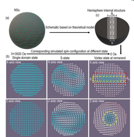
Fig. 2 Schematic representation of the micromagnetic simulations for the spin configuration in NSs (a and b) and the corresponding cross-sectioned hemisphere (c) showing the curling vortex internal state.
