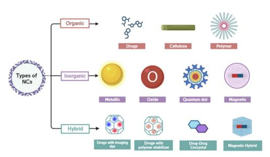
Fig. 1 Types of nanocrystals; figure is created with https://www.BioRender.com
