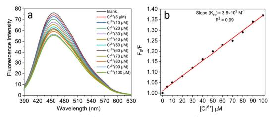
Fig. 4 (a) Fluorescence spectra of CNPs (2.0 mg mL $^{-1}$ ) in the presence of different amounts of Cr $^{6+}$  from the top to bottom: 5, 10, 20, 30, 40, 50, 60, 70, 80, 90, and 100  $\mu$ M in double-distilled water ( $\lambda_{\rm exc}=370$  nm) and (b) plot of  $F_0/F$  against the concentration of Cr $^{6+}$  (Stern–Volmer quenching response) at 454 nm.
