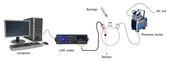
Fig. 1 Gas sensing setup.
