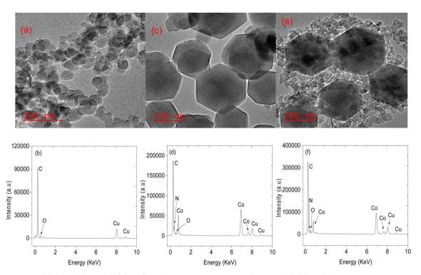
Fig. 3 TEM images of (a) CNPs, (c) ZIF-67 (e) CNPs/ZIF-67 and their respective EDS spectra, (b), (d) and (f).
