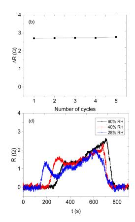
Fig. 8 (a) Repeatability of the CNPs/ZIF-67 sensor on acetone vapour, (b) its maximum amplitude of the response peaks and (c) a capacitance transient response repeatability test of the sensors, (d) acetone vapour relative response at different relative humidities and (e) transient acetone vapour response at different relative humidities.
