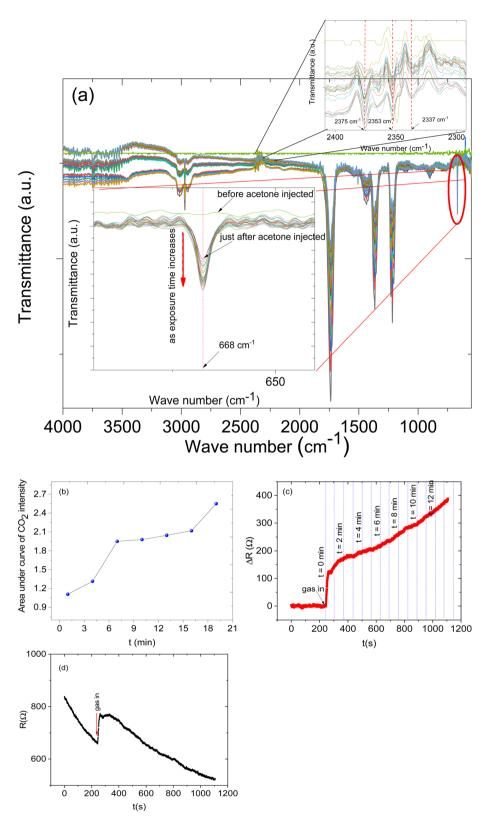
Fig. 10 (a) In situ FTIR: (b) areas under the curve of the CO<sub>2</sub> IR intensities against time (selected) (min), (c) the relative response of the sensor during the in situ FTIR coupled with LCR meter measurement and (d) transient response of the sensor during the in situ FTIR coupled with LCR meter measurement.
