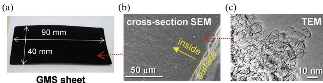
Fig. 8 (a) Photograph, (b) SEM and (c) TEM images of GMSs.<sup>58</sup> [This figure has been adapted/reproduced from ref. 58 with permission from the Royal Society of Chemistry, copyright 2019.]
