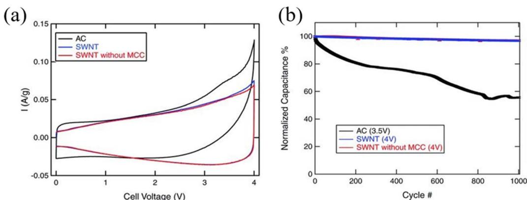
Fig. 6 (a) Cyclic voltammetry curves of AC, SWCNTs, and SWCNTs without MCC measured at  $1 \text{ mV s}^{-1}$  and (b) cycle stability over 1000 cycles at  $1 \text{ A g}^{-1}$ .<sup>51</sup> [This figure has been adapted/reproduced from ref. 51 with permission from John Wiley and Sons, copyright 2010.]
