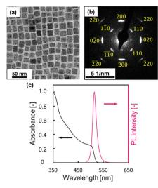
Fig. 1 (a) Schematic TEM image, (b) SAED pattern, and (c) optical properties of DDAB-covered CsPbBr<sub>3</sub> NCs.
