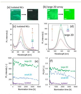
Fig. 3 (a and b) Changes in PL and (c and d) PL spectra of isolated NCs and large 2D arrays of CsPbBr<sub>3</sub> NCs under illumination at 450 nm; (e and f) time courses of Pl intensity and the PLQY of small and large 2D arrays and isolated NCs under illumination at 450 nm.
