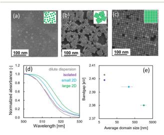
Fig. 2 (a-c) SEM images with schematic illustrations, (d) UV absorption edges, and (e)  $E_q$  as a function of the domain size in NC arrays; (a) isolated NCs, (b) small 2D arrays, and (c) large 2D arrays.
