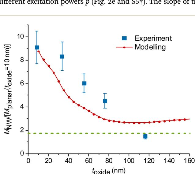
Fig. 4 Experimental and modelled excitation enhancement for  $\lambda = 640$  nm as a function of  $t_{\text{oxide}}$ . A  $M_{\text{planar}}$  reference for  $t_{\text{oxide}} = 10$  nm is assumed here. For the experiments, we used GaP NWs with  $d = 109 \pm 10$  nm. For the modelling, we assumed a fixed  $d = 110$  nm. Values above the dotted green line correspond to enhancement on the NW compared to a free fluorophore in water.
