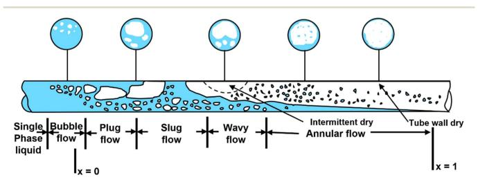
Fig. 7 Subcooled-inlet flow boiling patterns as a function of vapor quality (x) showing bubbly, plug, slug, wavy and annular flow followed by dryout.<sup>120</sup>
