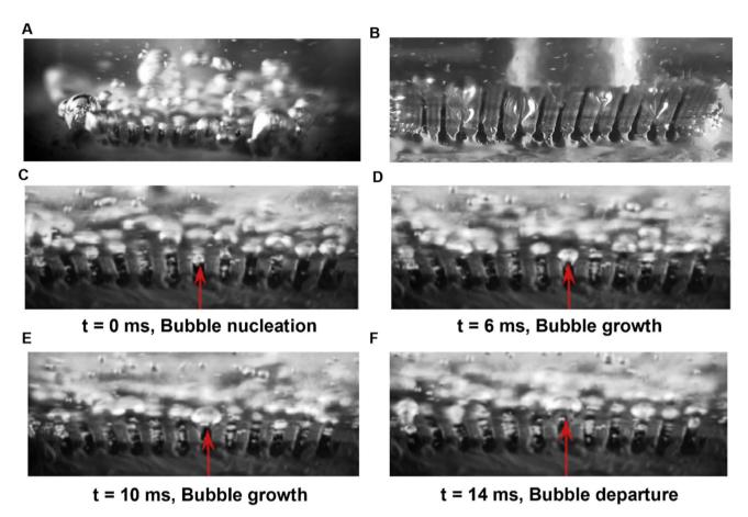
Fig. 4 Optical photograph demonstrating more nucleation for (A) porous structured reentrant cavity surface<sup>88</sup> when compared against (B) non-porous reentrant cavity surface with water as the working fluid.<sup>88</sup> (C–F) Bubble nucleation, growth and departure captured for porous reentrant cavity surface with ethanol as the working fluid.<sup>88</sup> Reproduced with permission from ref. 88. Copyright 2016 Elsevier.
