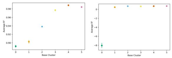
Fig. 10 Task transfer learning performance as average  $R^2$  value as a function of base generic cluster. On the left is transfer from hydrogen at 77 K to hydrogen at 243 K at 100 bar, and mirrors Fig. 7's non-task transfer results. On the right is transfer from hydrogen at 243 K to methane at 298 K. Note the change in scale of the vertical axis.
