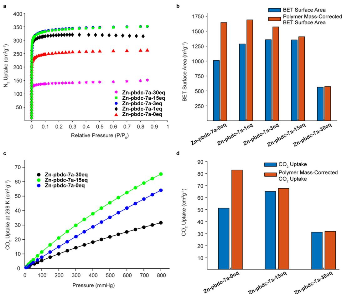
**Fig. 4**  $\text{N}_2$  (a) and  $\text{CO}_2$  (c) gas sorption isotherms for a series of polyMOF-5 materials synthesized from pbdc-7a and  $x$  equivalents of free  $\text{H}_2\text{bdc}$  linkers and a comparison of the polyMOFs' BET surface areas (b) and total  $\text{CO}_2$  uptake at 298 K and 1 atm (d). BET surface areas and  $\text{CO}_2$  uptake capacities corrected to only account for the mass contributing to the framework are shown in red.
