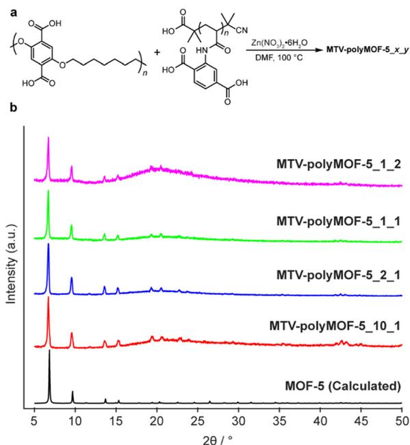
Fig. 5 (a) Synthesis of mixed polymer ligand polyMOFs MTV-polyMOF-5<sub>x</sub><sub>y</sub> from *x* equivalents of **pbdc-7a** and *y* equivalents of **pabdc-0a** and (b) powder X-ray diffractogram of series of MTV-polyMOF-5<sub>x</sub><sub>y</sub>.
