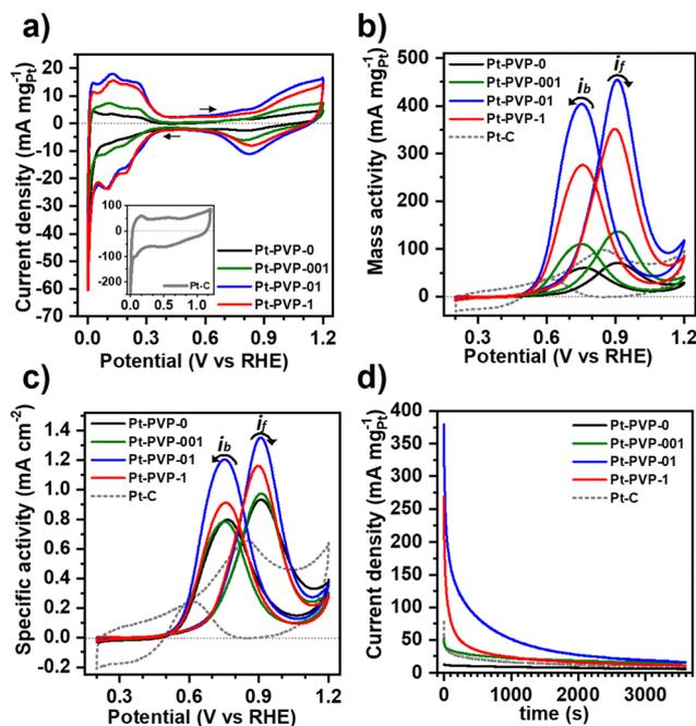
Fig. 3 (a) CVs of the different Pt NCs in 0.5 M H<sub>2</sub>SO<sub>4</sub> solution at  $50$  mV s<sup>-1</sup>, inset: CV of Pt/C. (b) and (c) mass activity and specific activity of the Pt NCs and Pt-C recorded in 0.5 M H<sub>2</sub>SO<sub>4</sub> + 1.0 M MeOH solution at  $50$  mV s<sup>-1</sup>. (d) Chronoamperograms of the different materials in 0.5 M H<sub>2</sub>SO<sub>4</sub> + 1.0 M MeOH solution at  $0.9$  V<sub>RHE</sub>. Arrows indicate the direction of the scan.
