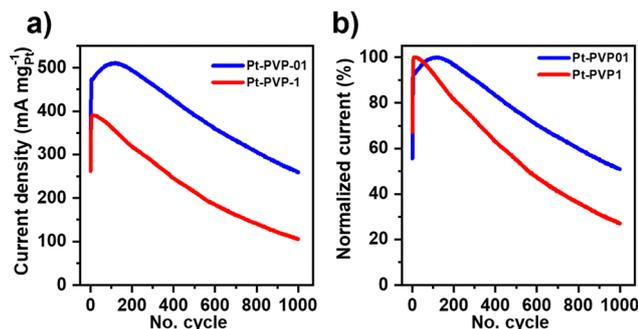
Fig. 4 Accelerated stability test (ADT) of Pt-PVP-01 and Pt-PVP-1 in 0.5 M H<sub>2</sub>SO<sub>4</sub> + 1.0 M MeOH solution at 50 mV s<sup>-1</sup>. (a) MA value at the  $i_f$ , (b) normalized data to the highest value.
