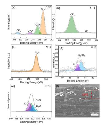
Fig. 5 XPS spectra of Li electrodes after cycling for 50 cycles: (a) C1s, (b) F1s, (c) N1s, (d) Li1s, and (e) O1s. (f) Cross-sectional SEM image of Li/rQPE/ LFP after cycling for 50 cycles.
