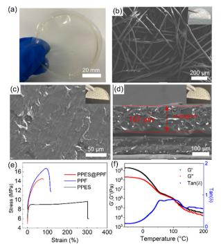
Fig. 2 (a) Optical photo of the as prepared PPES film. (b) SEM image of PPF from face mask. (c) Surface morphologies of PPES@PPF. The inset is the optical photo of the PPES@PPF film. (d) Cross-sectional SEM images of PPES@PPF. (e) Tensile test of PPES, PPF and PPES@PPF. (f) Temperature sweep of DMA of PPES. The blue line is the loss tangent  $\tan \delta$ ).
