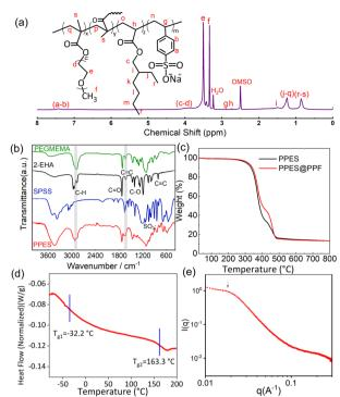
Fig. 1 Characterization studies of monomers and the as prepared polymer. (a) <sup>1</sup>H NMR spectra of the prepared PPES. (b) FT-IR spectra of PEGMEMA, SPSS, 2-EHA monomers and the resulting polymer network PPES. (c) The thermogravimetric analysis of PPES and PPES@PPF. (d) DSC curve of PPES. (e) SAXS spectrum of PPES.
