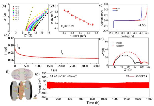
Fig. 3 (a) EIS curves of rQPEs from 25 °C to 60 °C. (b) The temperature-ionic conductivity fitted by Vogel-Fulcher-Tammann (VFT) behavior. (c) LSV curve of rQPE from 2.0-5.2 V. (d) Potentiostatic polarization curve with applied potential of 10 mV and (e) the corresponding EIS curves of symmetric cells. (f) Schematic illustration of Li<sup>+</sup> transport through the rQPE in Li/rQPE/Li symmetric cell. (g) Cycling performance of Li/rQPE/Li symmetric cell.
