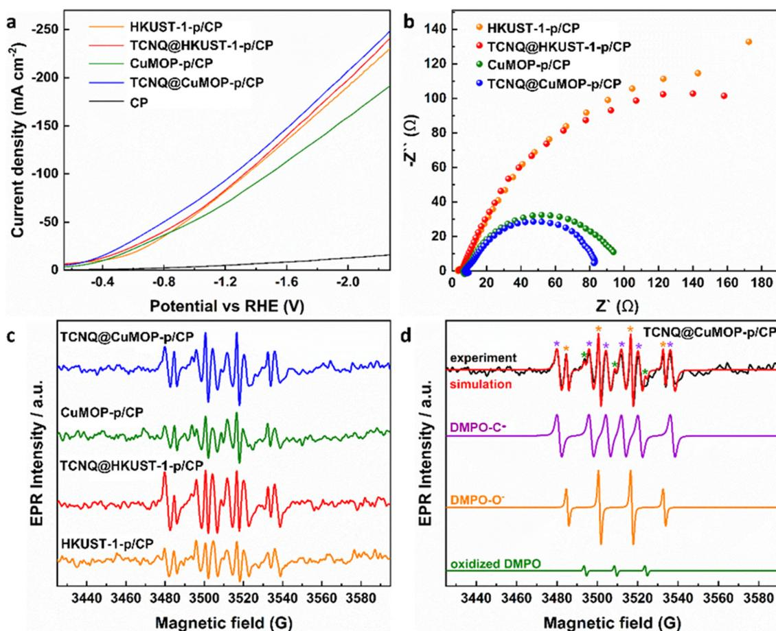
Fig. 5 (a) Linear sweep voltammetry (LSV) in  $\text{CO}_2$ -saturated electrolyte. (b) EIS spectra. (c) EPR spectra of electrolyte aliquots taken with different catalysts after electrolysis for 30 min. (d) EPR spectra of spin adducts of free radicals. The complete set of parameters for simulations are given in Tables S2 and S3 (ESI†).
