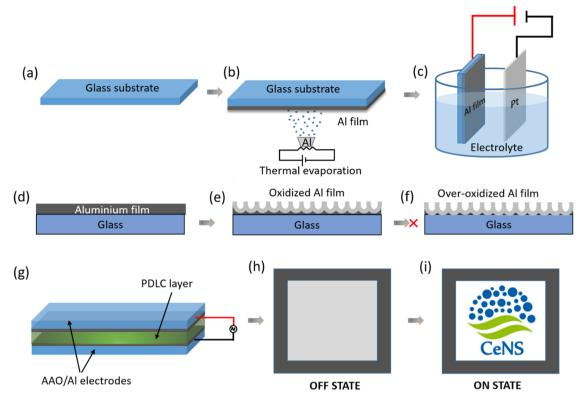
Fig. 1 Schematic illustration of (a-c) the deposition of the aluminium film and the anodization process setup, (d-f) the cross-sectional view of the Al film at different stages of the anodization process, (g) fabrication of the PDLC based smart window device using the anodized nanoporous aluminium (AAO/Al). (h) OFF or opaque state and (i) ON or transparent state of the PDLC smart window.
