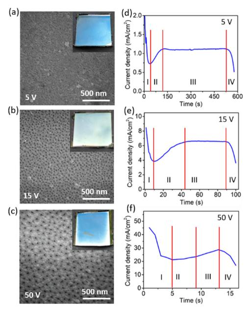
Fig. 2 FESEM images of the anodized nanoporous aluminium (AAO/AI) film at anodization voltages of (a) 5 V (b) 15 V and (c) 50 V. Inset images: photograph of the films, showing uniformity of the anodized film. Current density profile during anodization process at different applied anodization voltages of (d) 5 V (e) 15 V and (f) 50 V
