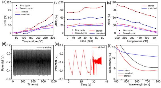
Fig. 4 Temperature stability test for the etched and unetched AAO/Al TCE. Relative change in resistance (ΔR/R) with increasing the temperature up to 300 °C (a), at the temperature 300 °C for 60 minutes (b), decreasing the temperature from 300 °C to ambient temperature (c). Electrochemical cyclic stability test for the unetched (d) and etched AAO/Al TCE (e). (f) Reflectance comparison between glass and the AAO/Al TCEs
