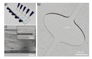
Fig. 2 a) Photograph of a sealed and connected chip incorporating five individual channels. b) Focus stack image of the imprinted channel structure into 240 µm thick COC. c) Image of the cross-section of a microfluidic channel sealed with a 2 mm thick COC slide by the solvent-assisted bonding technique (the inset shows the channel at higher resolution).
