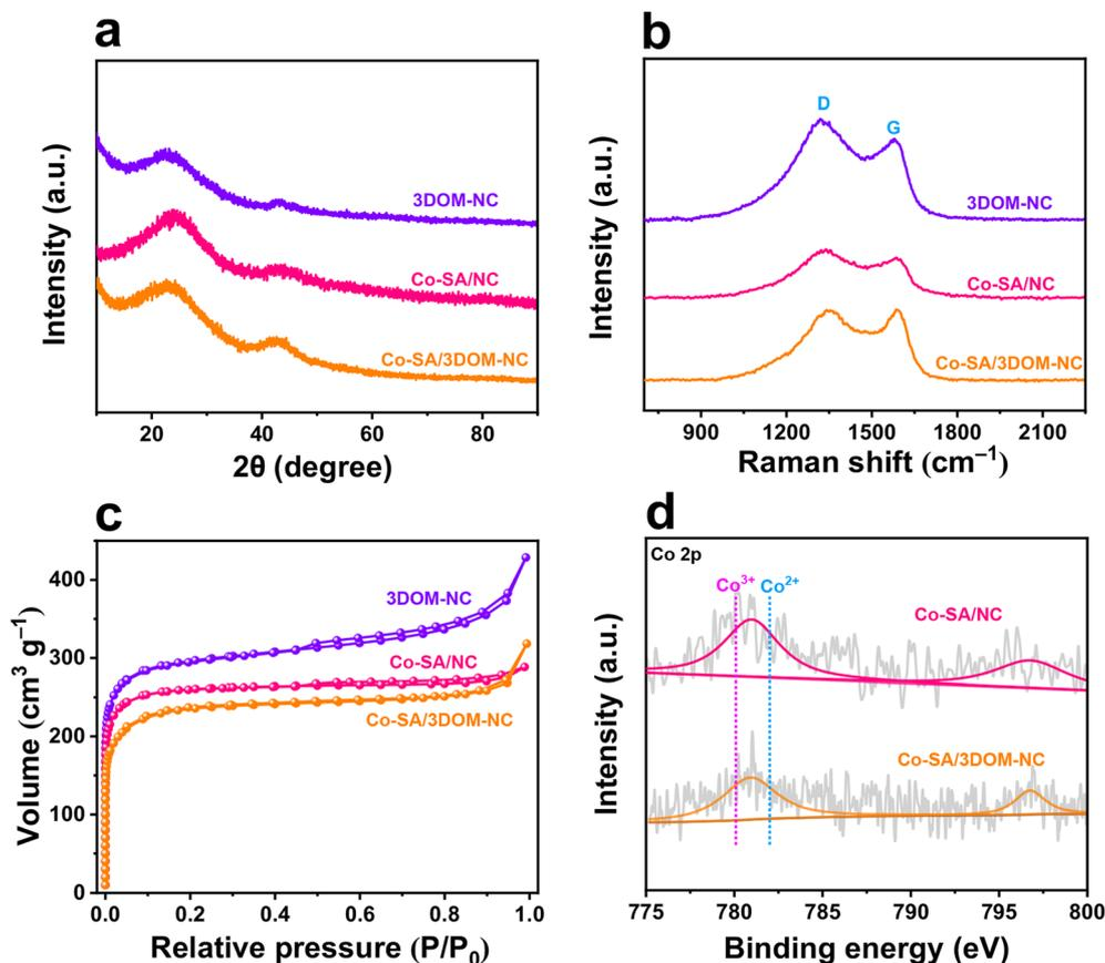
Fig. 3 (a) XRD patterns, (b) Raman spectra, and (c) N<sub>2</sub> adsorption-desorption isotherms of Co-SA/3DOM-NC, Co-SA/NC, and 3DOM-NC. (d) High-resolution Co 2p XPS spectra of Co-SA/3DOM-NC and Co-SA/NC.
