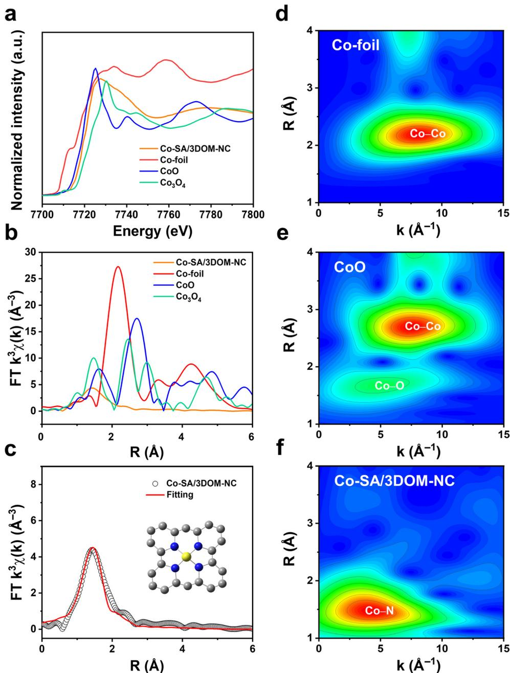
Fig. 4 (a) XANES spectra and (b) Fourier-transform EXAFS spectra of Co-SA/3DOM-NC, Co foil, CoO, and  $\text{Co}_3\text{O}_4$ . (c) Fourier-transform EXAFS fitting curves of Co K-edge for Co-SA/3DOM-NC (inset: a proposed structural model of Co-SA/3DOM-NC). Wavelet-transformed contour plots of Co in (d) Co foil, (e) CoO, and (f) Co-SA/3DOM-NC.
