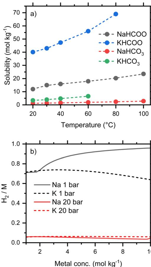
Fig. 4 (a) Solubilities of Na and K salts; (b) equilibrium conversion, expressed as the molar ratio of H<sub>2</sub> gas to metal, of aqueous Na and K formate/bicarbonate solutions between 1 and 10 mol kg<sup>-1</sup> at 60 °C.
