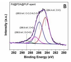
Fig. 12 High-resolution XPS spectra of the C 1s core level region of Pd@PDA@PUF: (A) as-synthesized, (B) spent (after 15 cycling tests).
