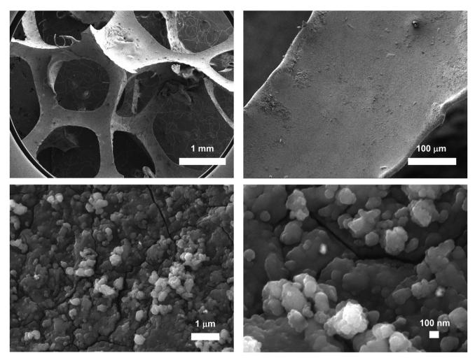
Fig. 2 HR-SEM images with different magnifications of the as-synthesized Pd@PDA@PUF.
