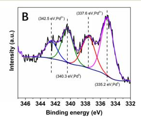
Fig. 11 High-resolution XPS spectra of the Pd 3d core level region of Pd@PDA@PUF: (A) after one run of semi-hydrogenation of phenylacetylene, (B) after one run of Suzuki coupling of bromobenzene and phenylboronic acid.
