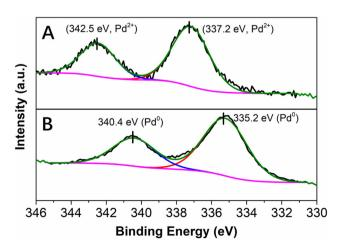
Fig. 4 High resolution XPS spectra of the Pd 3d core level region of Pd@PDA@PUF: (A) as-synthesized, (B) spent (after 15 cycling tests).
