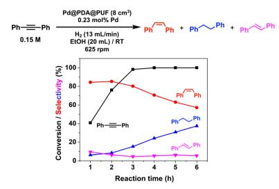
Fig. 8 Hydrogenation with Pd@PDA@PUF (8 cm<sup>3</sup>) of 1,2-diphenylacetylene; black squares: alkyne conversion; red circles, (Z)-alkene selectivity; blue triangles: alkane selectivity; pink triangle: (E)-alkene selectivity. Reaction conditions: 1,2-diphenylacetylene (3 mmol), Pd  $(7 \times 10^{-3} \text{ mmol})$ 0.23 mol%), EtOH (20 mL), H<sub>2</sub> flow rate (13 mL min<sup>-1</sup>), 25 °C, 625 rpm.
