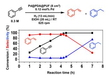
Fig. 5 Hydrogenation of phenylacetylene with Pd@PDA@PUF (8 cm<sup>3</sup>); black squares: PA conversion; red circles, ST selectivity; blue triangles: EB selectivity. Reaction conditions: PA (6 mmol), Pd  $(7 \times 10^{-3} \text{ mmol})$ , 0.12 mol%), EtOH (20 mL), H<sub>2</sub> flow rate (13 mL min<sup>-1</sup>), room temperature, 625 rpm.
