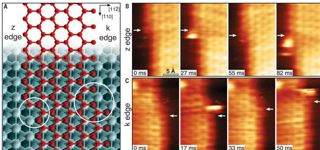
**Fig. 9** (A) Zigzag and Klein edges of a top-fcc epitaxial graphene layer on Ni (111). (B) High-speed STM sequence acquired at 710 K in quasi-constant height mode at the z edge. White arrows indicate the position of C atoms in fcc-hollow sites near the kink. (C) Same as in (B) but for the k edge. Reproduced with permission.<sup>68</sup> Copyright © 2018, The Authors.
