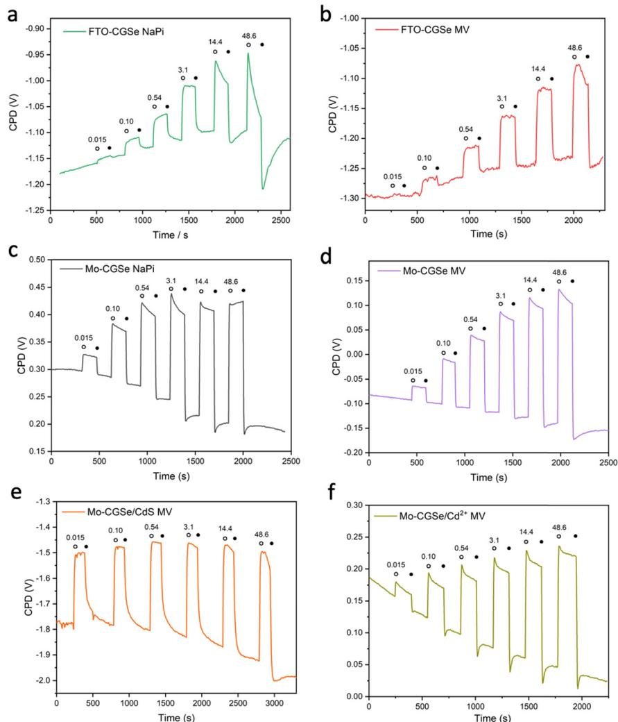
Fig. 5 Surface photovoltage (SPV) data as a function of light intensity ( $\text{mW cm}^{-2}$ ) from a 400 nm LED. (a) FTO-CGSe/NaPi, (b) FTO-CGSe/MV, (c) Mo-CGSe/NaPi, (d) Mo-CGSe/MV, (e) Mo-CGSe/CdS/MV, and (f) Mo-CGSe/Cd<sup>2+</sup>/MV.
