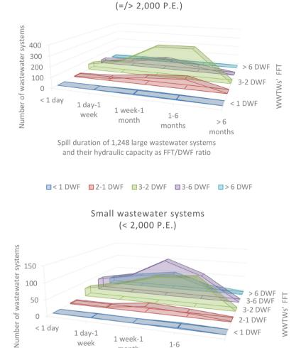
Spill duration of 726 small wastewater systems and their hydraulic capacity as FFT/DWF ratio □ < 1 DWF □ 2-1 DWF □ 3-2 DWF □ 3-6 DWF □ > 6 DWF
