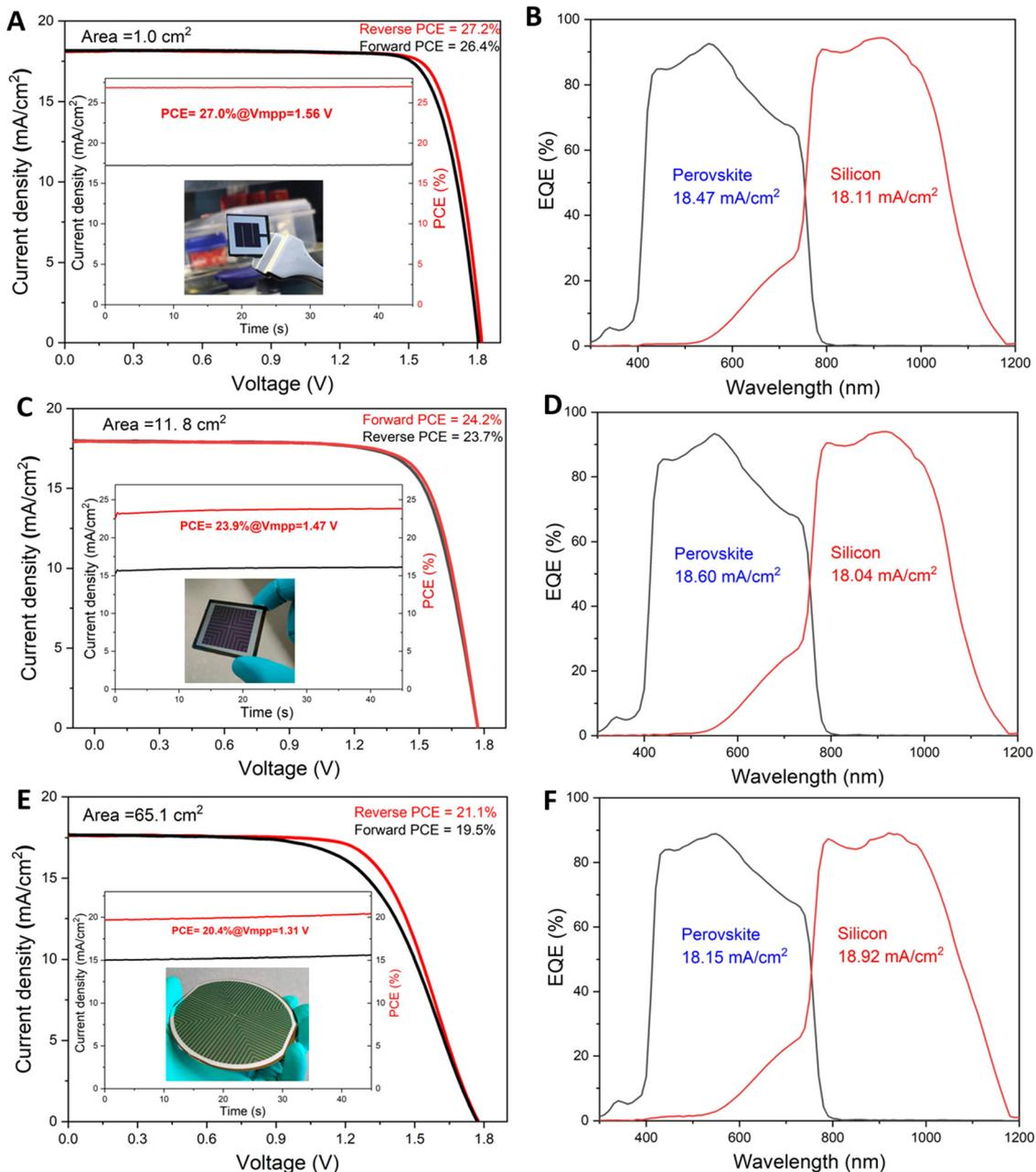
Fig. 4 Performance of champion tandem devices of different sizes. (A, C and E) light  $J$ - $V$  and (B, D and F) external quantum efficiency (EQE) of the perovskite-Si tandem devices of (A and B)  $1\text{ cm}^2$ , (C and D)  $11.8\text{ cm}^2$ , and (E and F)  $65.1\text{ cm}^2$ . Insets show the photographs of the fabricated tandem devices and their steady-state current densities and steady-state PCEs at fixed voltages near their maximum power points.
