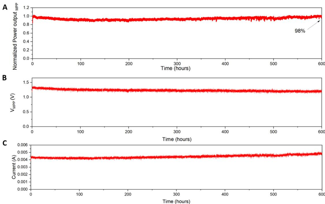
**Fig. 5** Stability testing of encapsulated 1 cm<sup>2</sup> perovskite-Si tandem cells under continuous illumination (100 mW cm<sup>-2</sup>) at relative humidity of 60 ± 20% at room temperature. Maximum power point tracking of (A) power output, (B) voltage (V<sub>MPP</sub>) at the maximum power point and (C) current to the starting value at the maximum power.
