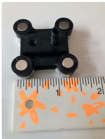
Fig. 1 (a) Schematic diagram of a prototype micro aerosol sampler. (b) 3D rendition of the tapered inlet. (c) Photo showing a 3D-printed micro-sampler. The ruler is on the cm scale.
