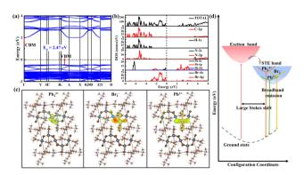
Fig. 4 (a) Calculated electronic band structures and (b) DOS of (HM)Pb<sub>2</sub>Br<sub>6</sub>. (c) Calculated charge density for (HM)Pb<sub>2</sub>Br<sub>6</sub> (Pb<sub>2</sub><sup>3+</sup> STELs, Br<sub>2</sub><sup>-</sup> and Pb<sup>3+</sup> STHLs holes) upon crystal lattice perturbation via the Pb-Pb, Br-Br and Pb-Br distances shortening. (d) Configuration coordinate diagram illustrating the luminescence mechanism.
