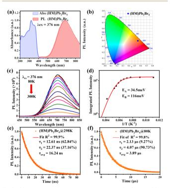
Fig. 2 (a) Normalized absorption and PL spectra of (HM)Pb<sub>2</sub>Br<sub>6</sub>. (b) The CIE 1931 chromaticity coordinate. (c) Temperature-dependent PL spectra of (HM)Pb2Br6. (d) Integrated PL intensity as a function of reciprocal temperature. Time-resolved PL decay curve of (HM)Pb2Br6 under a 375 nm excitation laser line at (e) 298 K and (f) 80 K.
