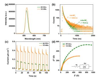
Fig. 3 (a) PL spectra and (b) time-resolved PL spectra of 3D NCs and 1D NRs powered counterparts (excitation: 405 nm laser). (c) Transient photocurrent responses and (e) EIS Nyquist plots of 3D NC and 1D NR electrodes under the same conditions (inset is the fitted equivalent circuit)
