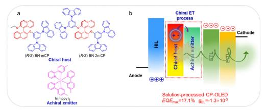
Fig. 1 (a) Molecular structure of the chiral host and achiral emitter; (b) schematic diagram of the solution processable CP-OLED.
