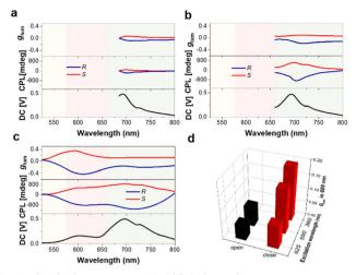
Fig. 4 (a-c) CPL spectra of R(S)-1-C-NR-Cy5 cholesteric texture ( $\lambda_{\rm ex}$  = 625 nm,  $\lambda_{\rm ex}$  = 550 nm,  $\lambda_{\rm ex}$  = 360 nm, respectively). (d) 3D Column diagrams of CPL  $g_{\text{lum}}$  values obtained by irradiation of donor  $R-\mathbf{1}$  or acceptor dyes when CET was turned "on" and "off", respectively.
