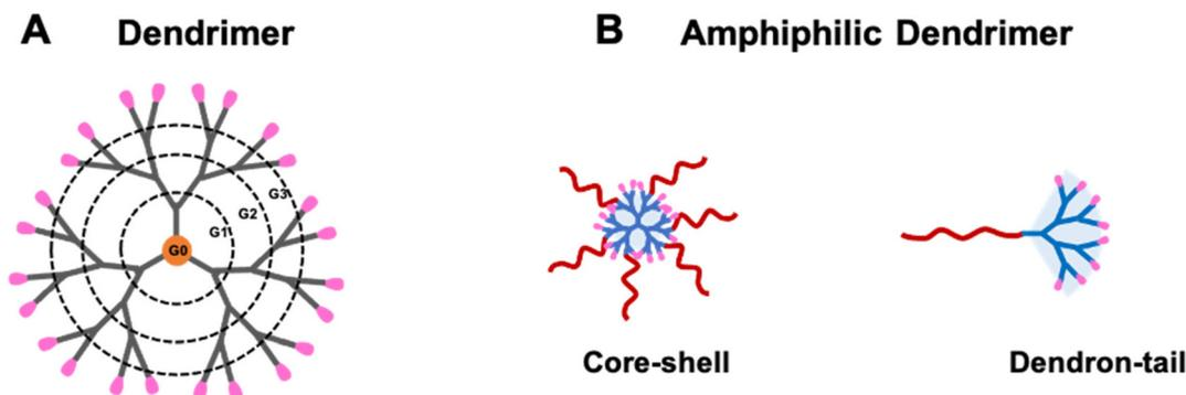
**Fig. 1** Cartoon illustrations of (A) a dendrimer and (B) amphiphilic dendrimers. (A) The dendrimer structure is composed of a central core, repeat branching units forming consecutive levels or generations (G1, G2 and G3) and terminal groups on the surface (shown in pink). (B) Amphiphilic dendrimers of core-shell and dendron-tail structures composed of distinct hydrophobic (red) and hydrophilic (blue) entities. Reproduced from ref. 30 with permission from ACS Publications, copyright 2023.
