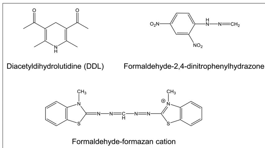
Fig. 5 Chromophores resulting from the reaction of formaldehyde with acetyl acetone (2,4-pentanedione), DNPH and MBTH.
