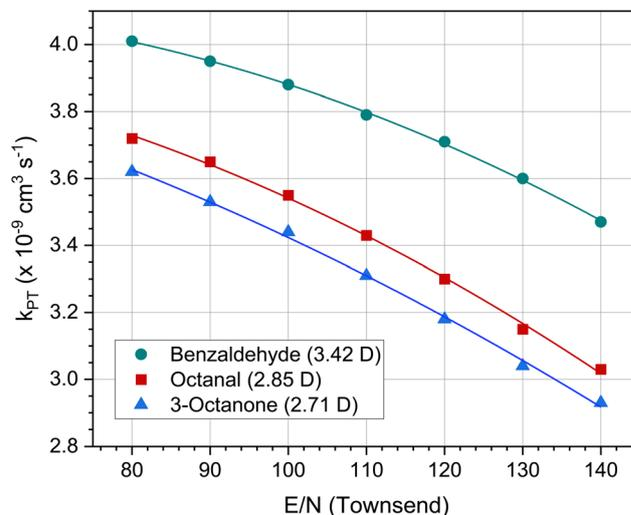
**Fig. 10** Dependence of the proton-transfer reaction constant *k<sub>PT</sub>* on the *E/N* ratio (electric field to molecular density) set in the PTR-MS device at 353 K for benzaldehyde, octanal and 3-octanone. The values in brackets indicate the respective dipole moment in Debye. The data were taken from Salthammer *et al.*<sup>135</sup>
