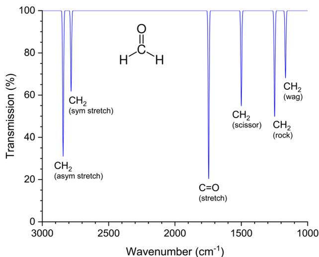
Fig. 3 Simulated IR spectrum of formaldehyde in the gas phase. The wavenumbers of the six normal modes were taken from the publication by Nakanaga *et al.*<sup>50</sup> The terms in brackets refer to different types of molecular vibrations (*sym stretch*: symmetrical stretching; *asym stretch*: antisymmetrical stretching; *stretch*: linear stretching; *scissor*: scissoring or bending, *rock*: rocking; *wag*: wagging).
