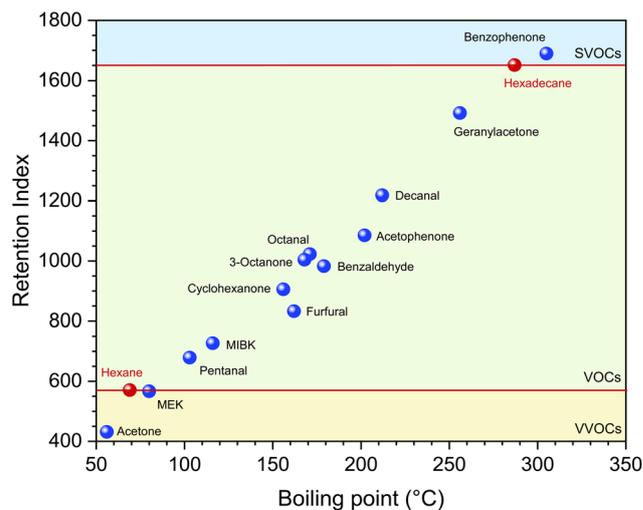
Fig. 7 Gas chromatographic retention indices of several carbonyl compounds *versus* boiling point in comparison to *n*-hexane and *n*-hexadecane. The indices were determined against a series of alkanes using a laboratory-specific method for non-isothermal conditions.<sup>88</sup>
