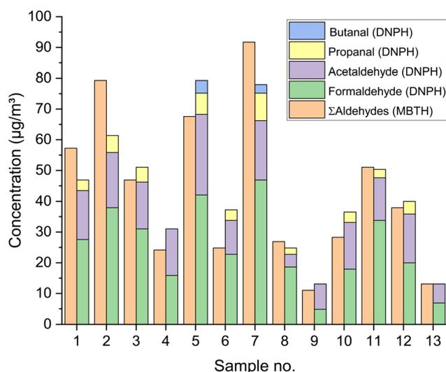
Fig. 6 Results of aldehyde measurements with DNPH and MBTH in test chambers on 13 different materials. Experimental details and data are published by Giesen *et al.*<sup>73</sup>
