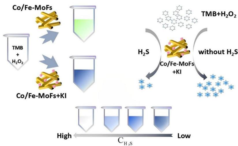
Fig. 19 Schematic illustration of  $\text{H}_2\text{S}$  detection by Co/Fe-MOFs- $\text{I}^-$  nanozyme-based colorimetric sensors.<sup>151</sup>
