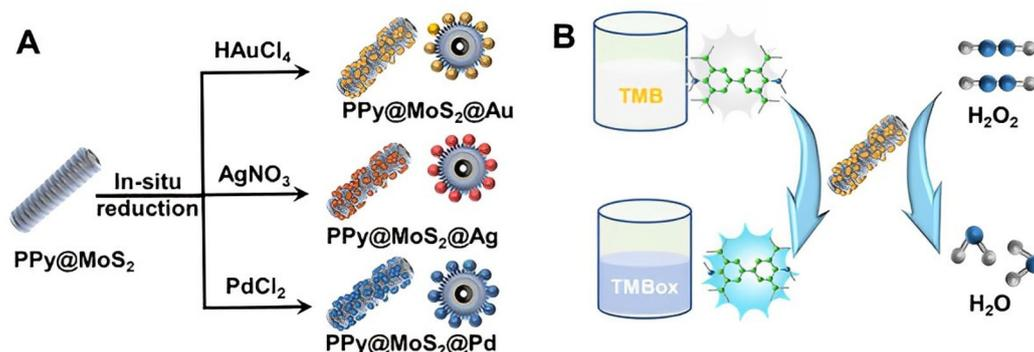
Fig. 9 (A) Schematic illustration of Au, Ag, and Pd NP-decorated PPy@MoS<sub>2</sub> nanocomposites prepared by *in situ* reduction and (B) PPy@MoS<sub>2</sub>@Au catalytic oxidation of TMB.<sup>114</sup>
