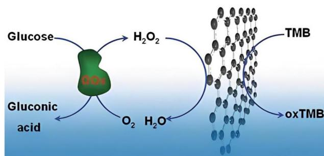
Fig. 11 Schematic diagram of a colorimetric approach for the detection of glucose based on GOx and the GO-COOH catalyzed TMB-H<sub>2</sub>O<sub>2</sub> system.<sup>122</sup>
