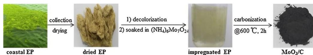
Fig. 17 Preparation of MoO<sub>3</sub>/C nanorods by a green tide biomass template.<sup>144</sup>
