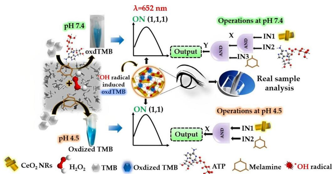
Fig. 7 Schematic illustration of the logic operation mechanism for melamine detection based on peroxidase-like activity of  $\text{CeO}_2$  NRs at acidic (4.5) and neutral (7.4) pH.<sup>103</sup>
