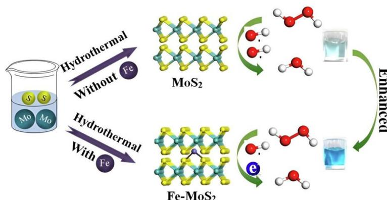
Fig. 8 Schematic diagram of enzyme activity comparison of  $\text{MoS}_2$  and Fe- $\text{MoS}_2$  prepared using a hydrothermal method.<sup>112</sup>
