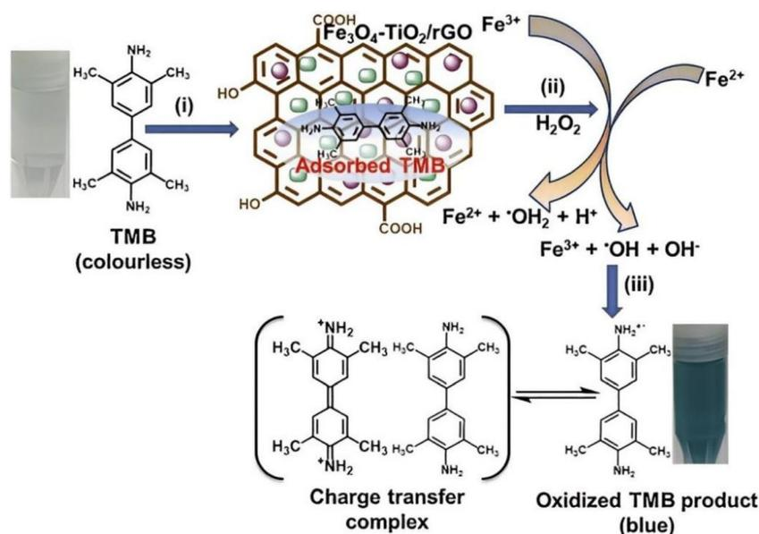
Fig. 13 Schematic illustration of (i) TMB adsorbed on the surface of Fe<sub>3</sub>O<sub>4</sub>-TiO<sub>2</sub>/rGO nanozymes, (ii)  $\cdot\text{OH}$  generated by the Fenton reaction, and (iii) TMB oxidized by  $\cdot\text{OH}$  radicals.<sup>127</sup>
