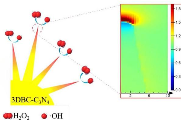
Fig. 14 Schematic diagram of the 3DBC-C<sub>3</sub>N<sub>4</sub> nanozymes accelerating electron collection in the tip region to activate H<sub>2</sub>O<sub>2</sub> to produce  $\cdot\text{OH}$ .<sup>135</sup>
