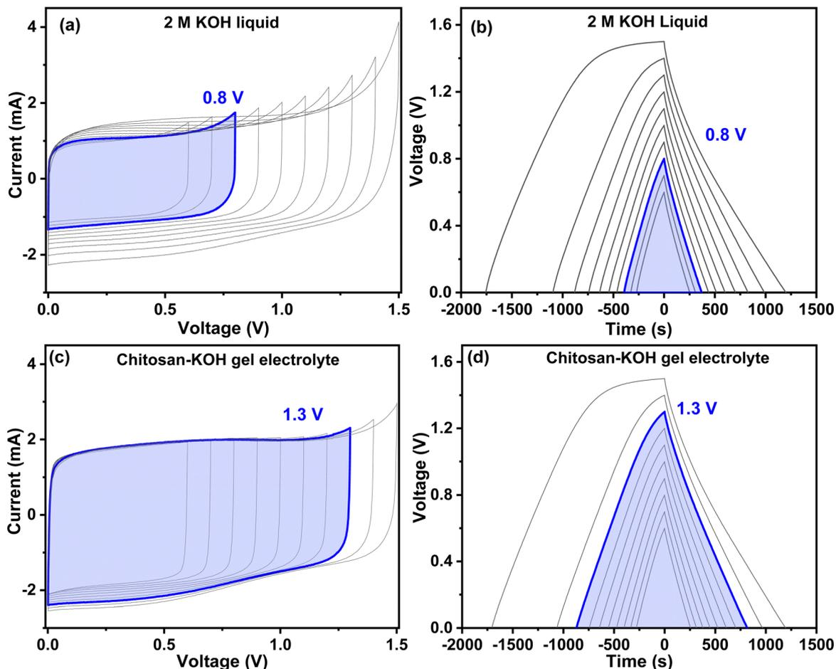
Fig. 7 (a) Cyclic voltammety at  $0.1 \text{ mV s}^{-1}$ , (b) galvanostatic charge discharge at  $0.1 \text{ A g}^{-1}$  of activated carbon using liquid 2 M KOH from 0.6 to 1.5 V, (c) cyclic voltammety at  $0.1 \text{ mV s}^{-1}$  and (d) galvanostatic charge discharge at  $0.1 \text{ A g}^{-1}$  using chitosan-KOH gel electrolyte.
