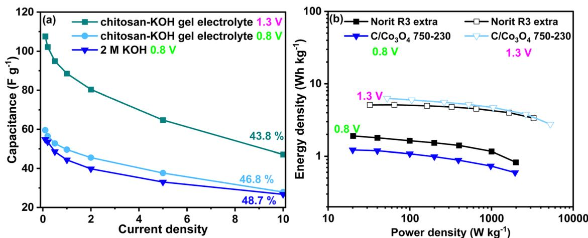
Fig. 10 Electrochemical performance of C/Co<sub>3</sub>O<sub>4</sub> 750–230 nanocomposite using chitosan–KOH gel electrolyte: (a) rate capability for 2 M KOH at 0.8 V and for chitosan–KOH gel electrolyte at 0.8 and 1.3 V, (b) Ragone diagram of C/Co<sub>3</sub>O<sub>4</sub> 750–230 nanocomposite and Norit R3 extra using 2 M KOH at 0.8 V and chitosan–KOH gel electrolyte at 1.3 V.
